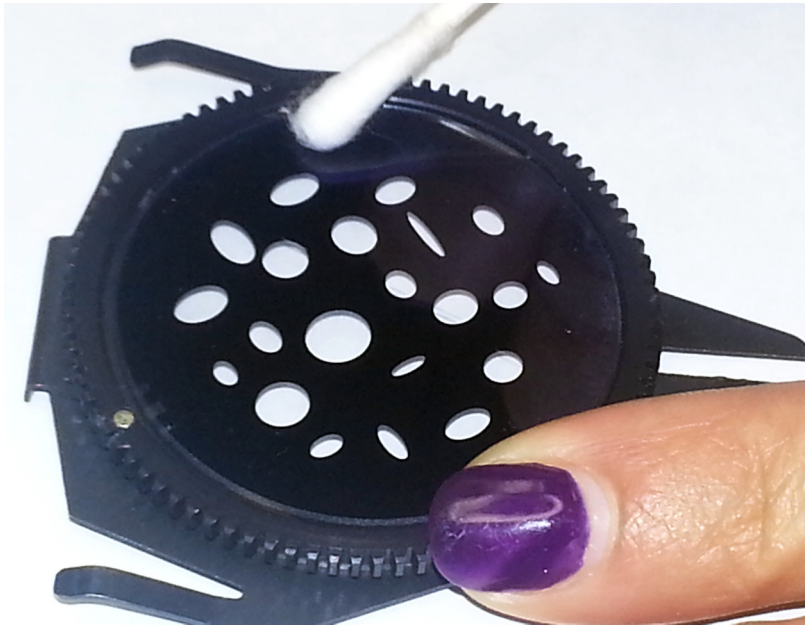
Figure 4: Securing Glass in Carrier
